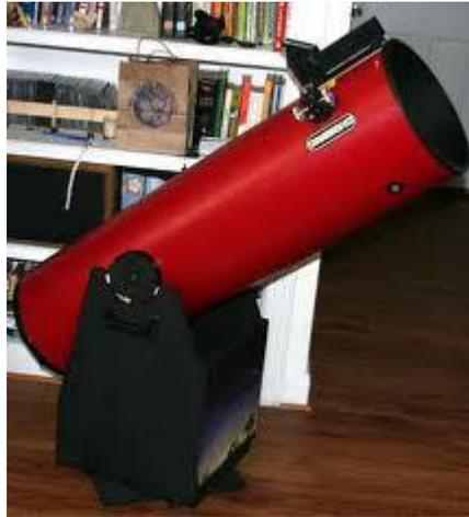
This instrument is twin to our loaner telescope, “Big Red,” a 13-inch Newtonian reflector, mounted in the Dobsonian style and originally used at Eagle Valley Middle School
